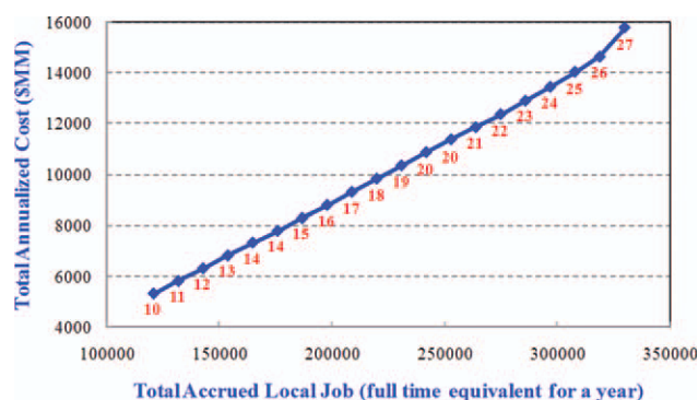
Figure 14. Pareto curve showing tradeoff between economic and social performances for case study 2 (numbers below the dots are for the optimal number of biorefinery plants to be installed in each Pareto curve solution).
